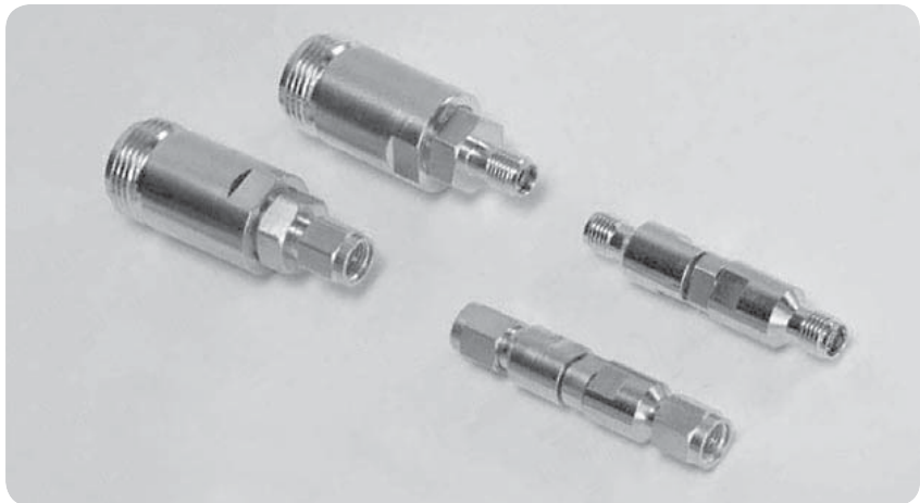
Figure 6. For millimeter-wave applications, the most common connector savers will have female connectors on both ends. Shown here are adapters to connect an analyzer with 2.4 mm front panel connectors to type-N and 2.4 mm accessories.
