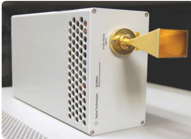
Figure 4. Agilent millimeter frequency ultra-wideband downconverter. The waveguide input with a horn antenna is at the upper right. This downconverter is driven by an external microwave local oscillator and its output is fed to an external digitizer such as an oscilloscope.
