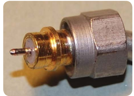
Figure 7. Figure 7a shows a 2.4 mm-to-3.5 mm adapter with the 2.4 mm end of the adapter on the right. The male connector at right is an SMA. The SMA male connector in Figure 7b has a non-captive nut and a male conductor which is displaced axially (too long) and is slightly bent, perhaps from the bending of the semi-rigid cable adjacent to the connector.
